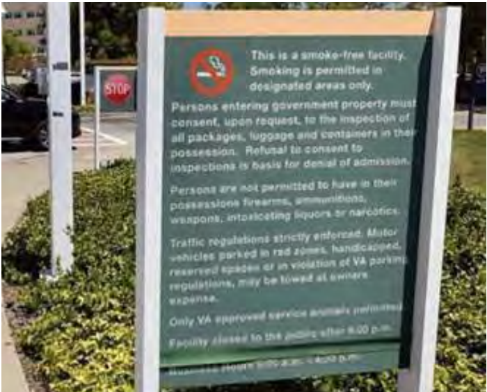
Figure 10.2.17-58. Mandatory policy signs at roadways are difficult to read from a vehicle due to small text size and colors.
