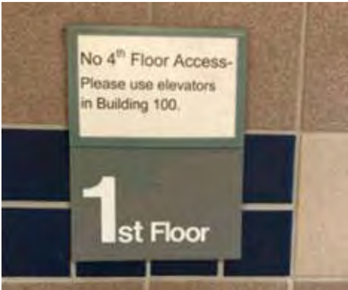
Figure 10.3.3-6. (PAD B100) Floor numbering identification would be simpler and more clear without “st,” “nd,” “rd,” and “th.” For instance, “Floor 1” rather than “1st Floor.”
