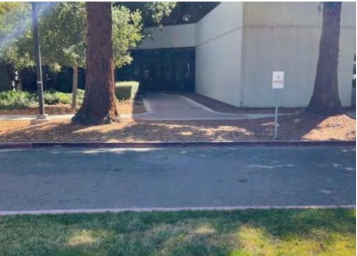
Figure 10.2.15-52. The route from parking to the closest, visible entrance of Building 334 at MPD does not have a direct, accessible route, nor any signage.
