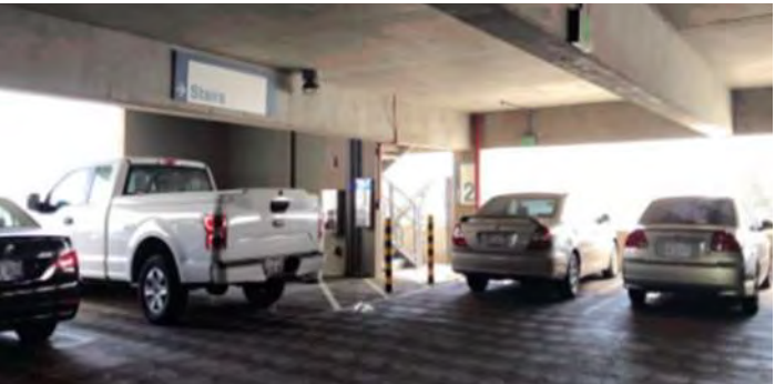
Figure 10.2.9-36. The stairs in this corner of PS1 don’t provide crucial wayfinding information. The stairway itself is unlabeled and there is no directional messaging telling users what they will find if they proceed up or down from this point.
