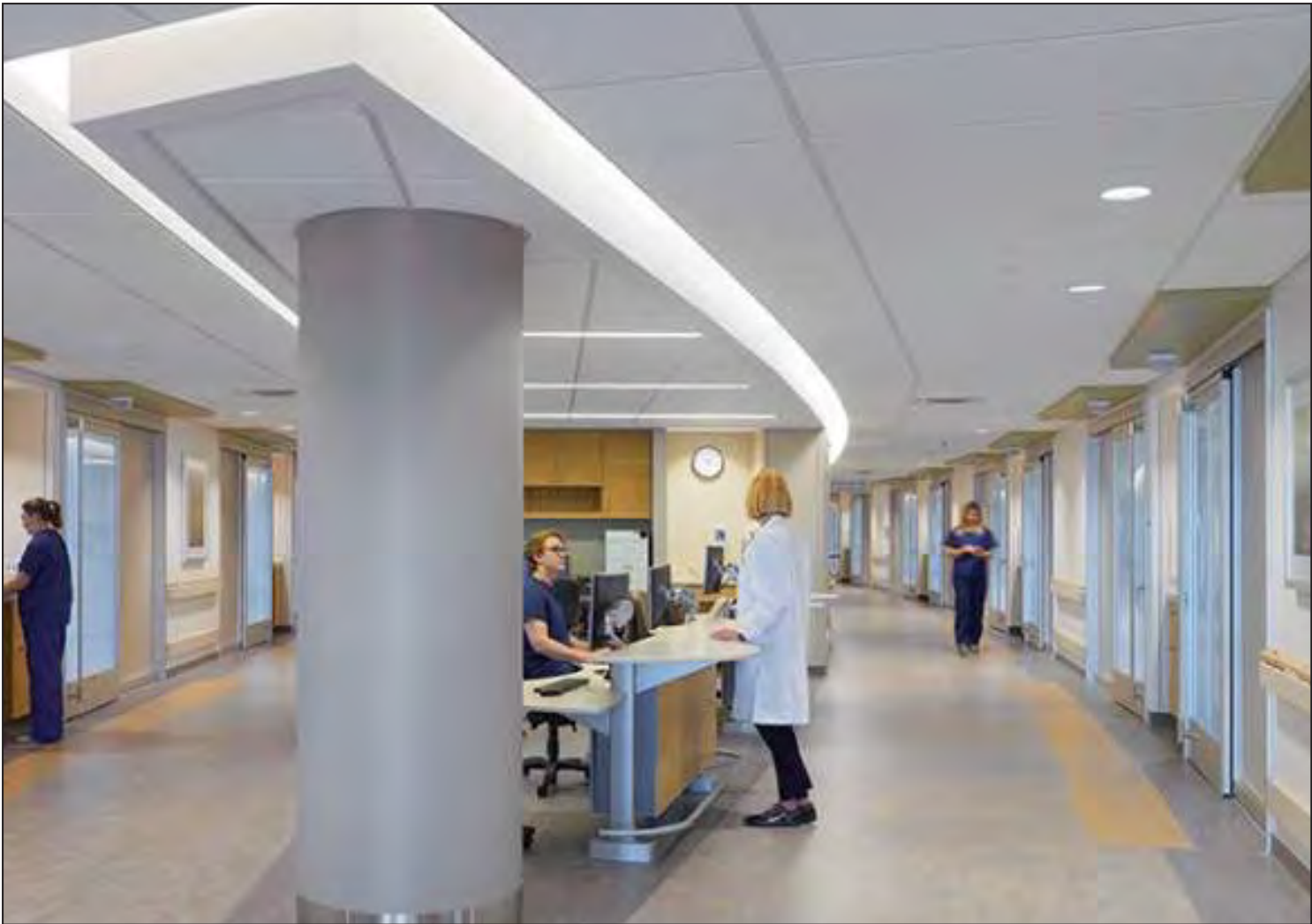
Figure 4.11-1. An example of using lighting to direct patients to a destination.
