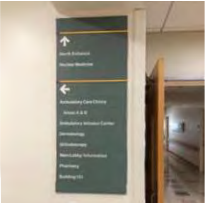
Figure 10.3.4-15. (PAD B100) This directional sign is too high. It should probably be divided into two, side-by-side directional signs. Sign messages are legible enough but we don't know about their accuracy. The sign would be more useful with location information in a header: building number, floor number.
