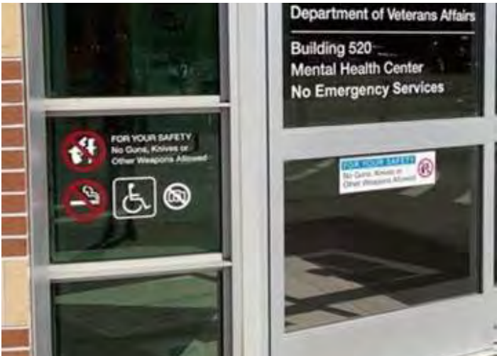
Figure 10.2.17-59. Use of icons for mandatory policies are more legible than long statutory text if they are recognizable to building users.
