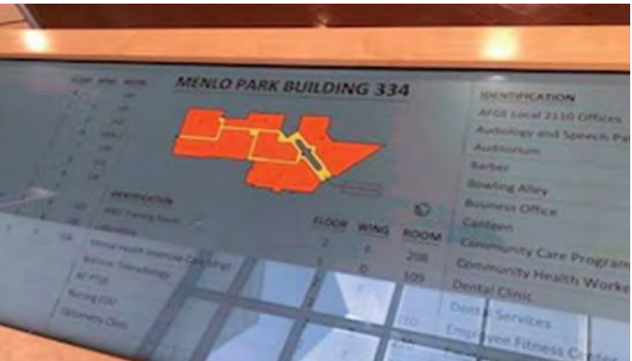
Figure 10.3.2-3. The building directory at B334 (MPD) is reflective, which makes it hard to read. Destinations are listed in an order that isn't easily discerned. The building map attached with the directory is out of date and is missing detailed information.
