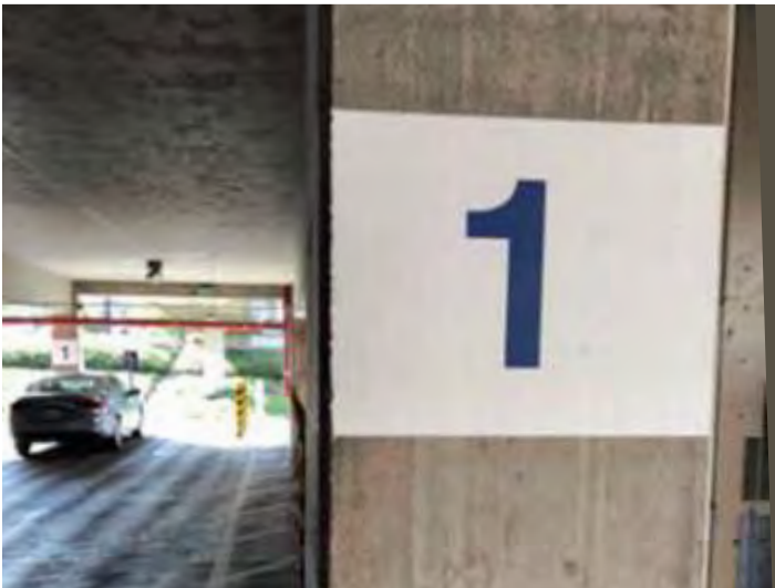
Figure 10.2.9-31. This sign is not useful because it is not clear that the “1” designates the garage level. The numeral is color coded but lacks indication for drivers that a color coding system is in use.
